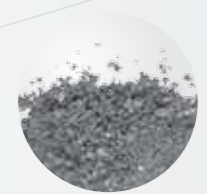
Biochar from sewage sludge Sterilized, odorless soil enhancer or solid fuel
